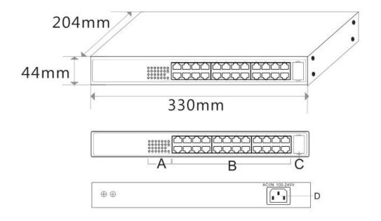
A.Working LED Indicator B.24\* POE port C.2\*gigabit SFP Port D.power input port:AC100-240.50-60HZ
