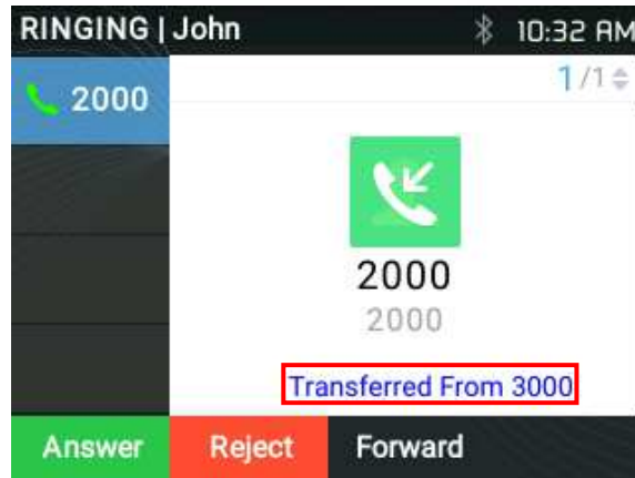
Figure 27: Transfer from Information While Ringing and During Incoming Call
