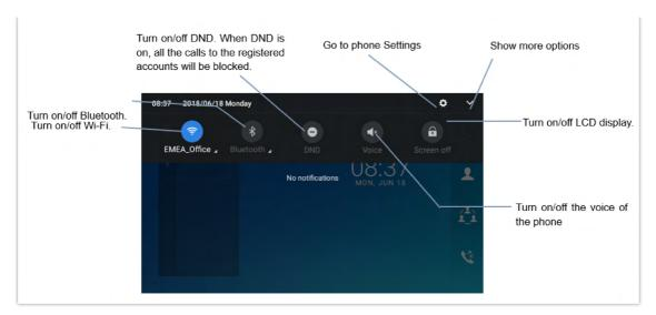
Figure 42: System Settings in Status Bar
