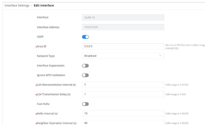
The screenshot shows the 'Edit Interface' configuration form for VLAN 10. The OSPF toggle is turned ON. The Area ID is set to 0.0.0.0. The Network Type is set to Broadcast. The LSA Retransmission Interval is 5, LSA Transmission Delay is 1, and the Hello Interval is 10. The Neighbor Expiration Interval is 40.
