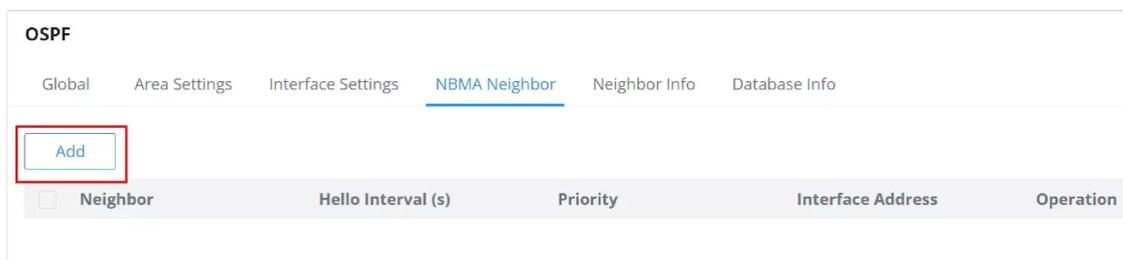
The screenshot shows the OSPF NBMA Neighbor configuration page. An 'Add' button is highlighted with a red box. Below it is a table with columns for Neighbor, Hello Interval (s), Priority, Interface Address, and Operation.
