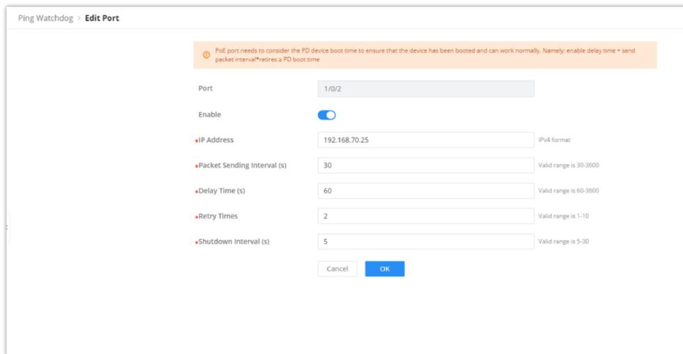
The screenshot shows the 'Ping Watchdog > Edit Port' configuration page. At the top, there is a warning message: 'Fail port needs to consider the PD device boot time to ensure that the device has been booted and can work normally. Namely: enable delay time + send packet interval \* retries > PD boot time'. Below this, the configuration fields are as follows:
