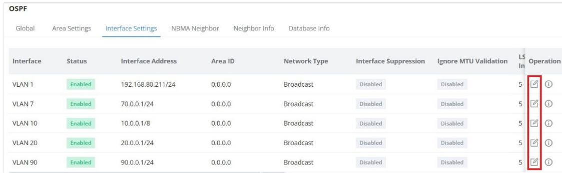
The screenshot shows the OSPF configuration page with the 'Interface Settings' tab selected. A table lists five interfaces: VLAN 1, VLAN 7, VLAN 10, VLAN 20, and VLAN 90. Each interface is currently 'Enabled'. The 'Operation' column for each interface contains an edit icon (pencil) and a refresh icon (circular arrow). A red box highlights the edit icons for all five interfaces.
