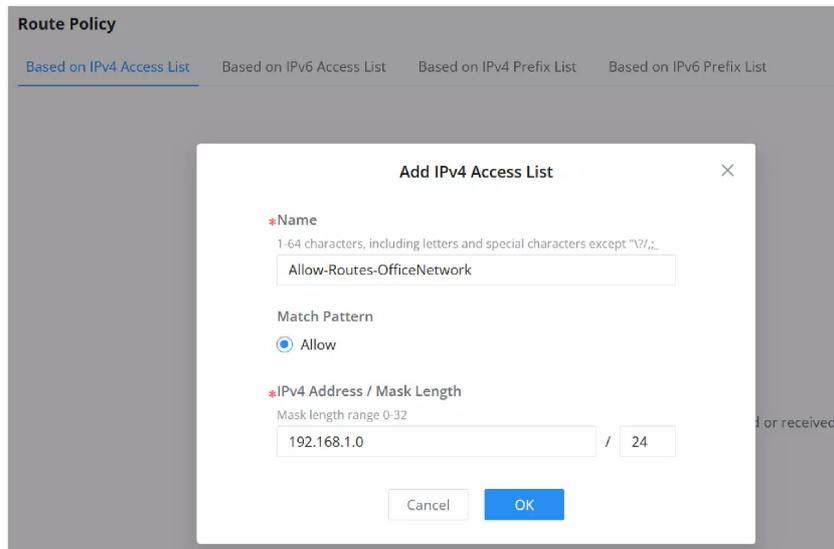
The screenshot shows the 'Route Policy' configuration page with four tabs: 'Based on IPv4 Access List', 'Based on IPv6 Access List', 'Based on IPv4 Prefix List', and 'Based on IPv6 Prefix List'. The 'Based on IPv4 Access List' tab is selected. A modal dialog box titled 'Add IPv4 Access List' is open, containing the following fields:
